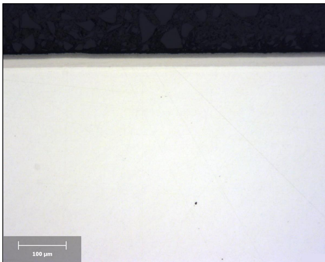
Figure 5: The coating layers after 3 µm polishing step– 100 x
