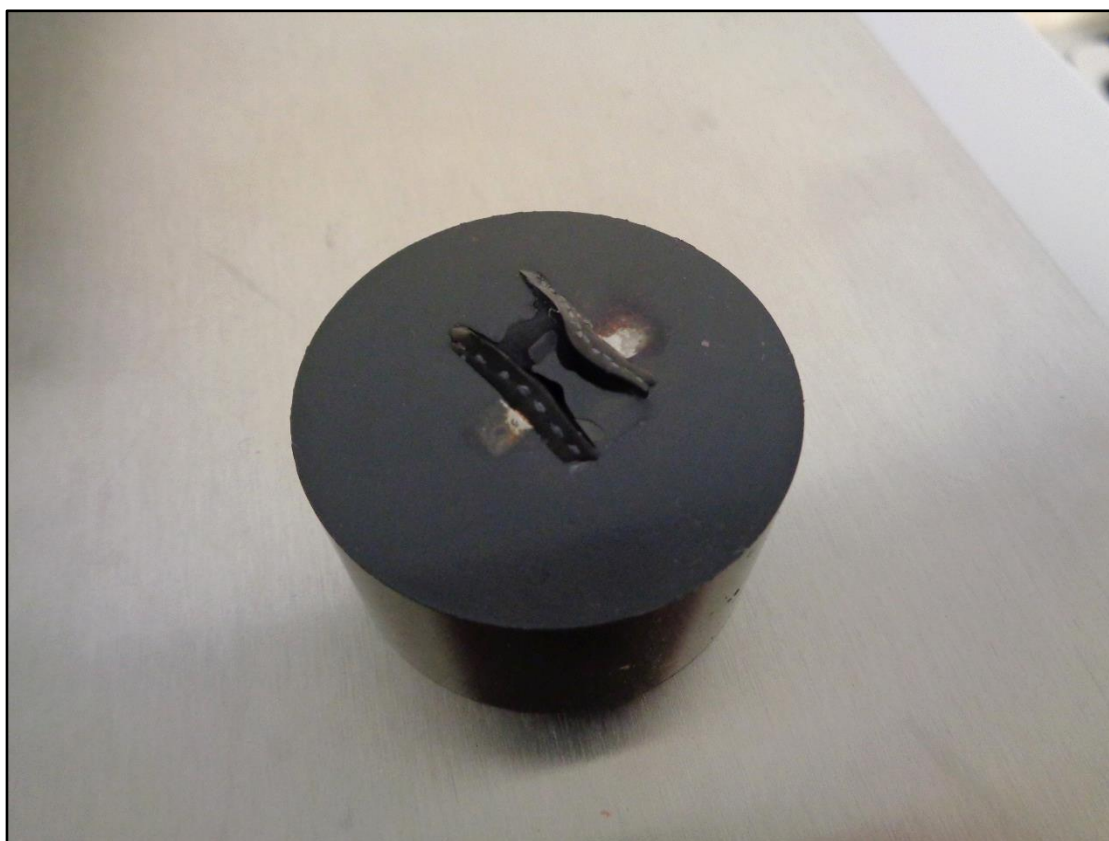
Figure 4: The mounted samples with plastic part which is not Ok.
