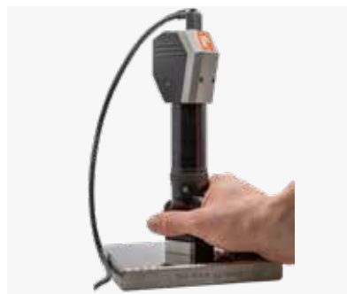
Indirect calibration using a hardness test block
