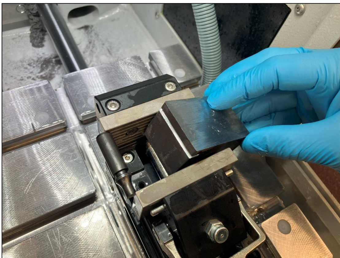
Figure 7: Clamping with support block.
