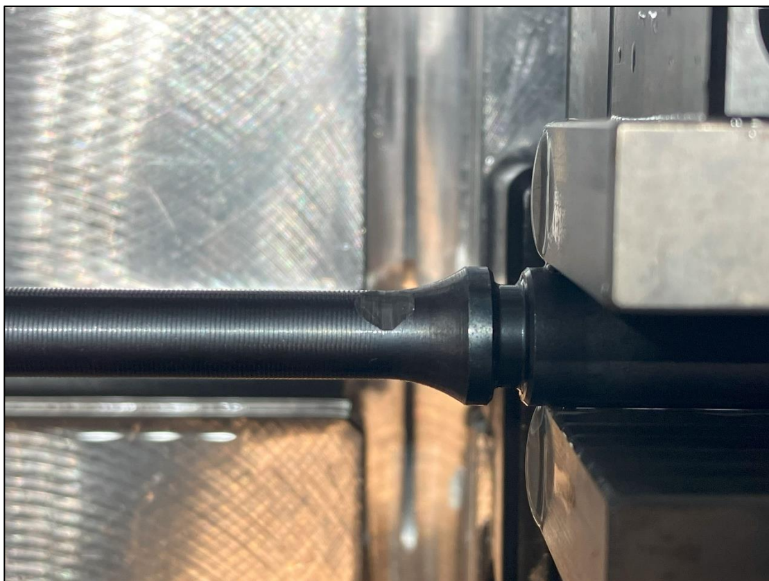
Figure 2: Failed cutting attempt with Type A.
