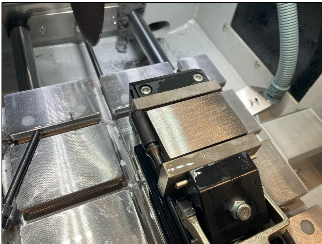
Figure 6: Clamping with support block.
