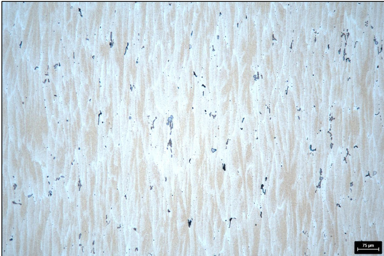
Figure 4: AA 7045 – etched – 200x.
