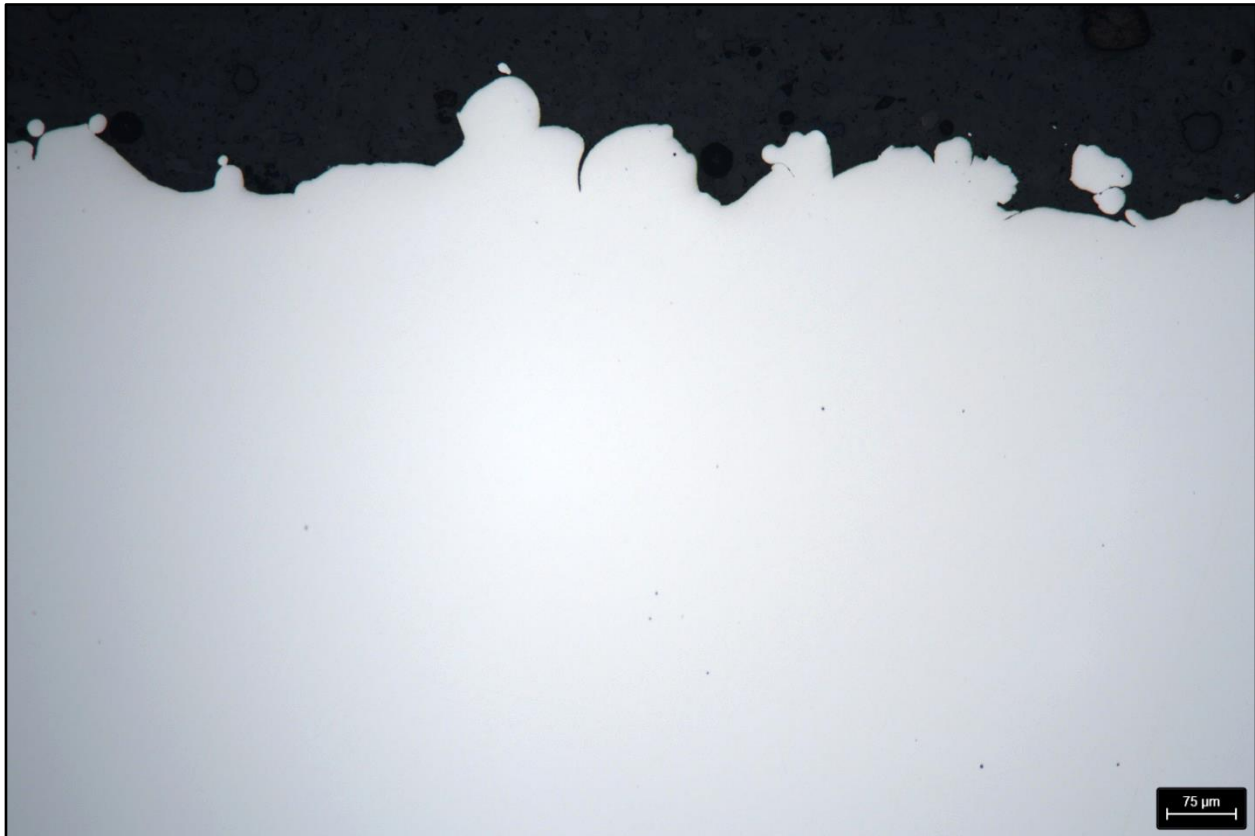
Figure 10: Maraging steel – unetched – 100x.
