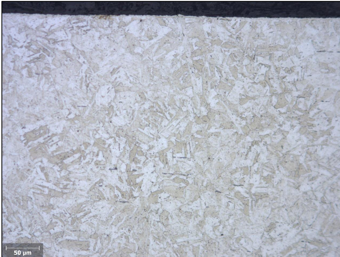
Figure 13: The microstructure after etching with Adler for 3 seconds – 200 x. Box B.
