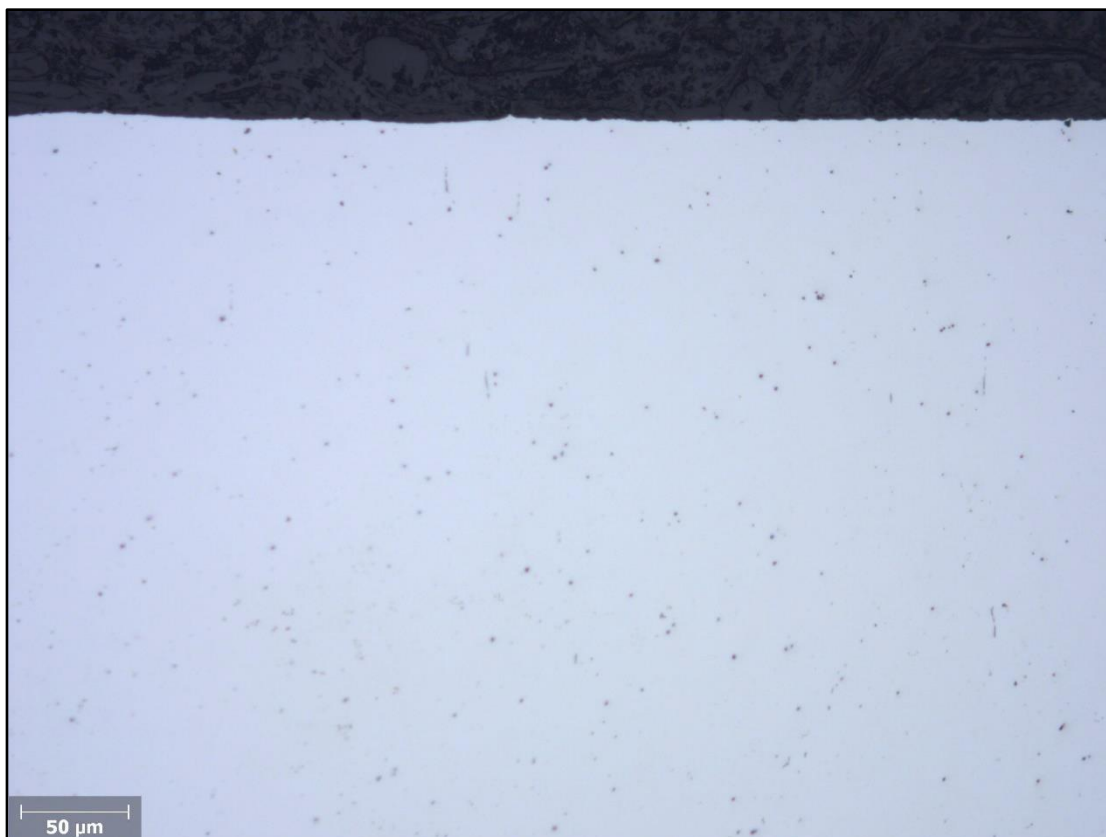
Figure 10: The microstructure after final polishing– 200 x. Box B.
