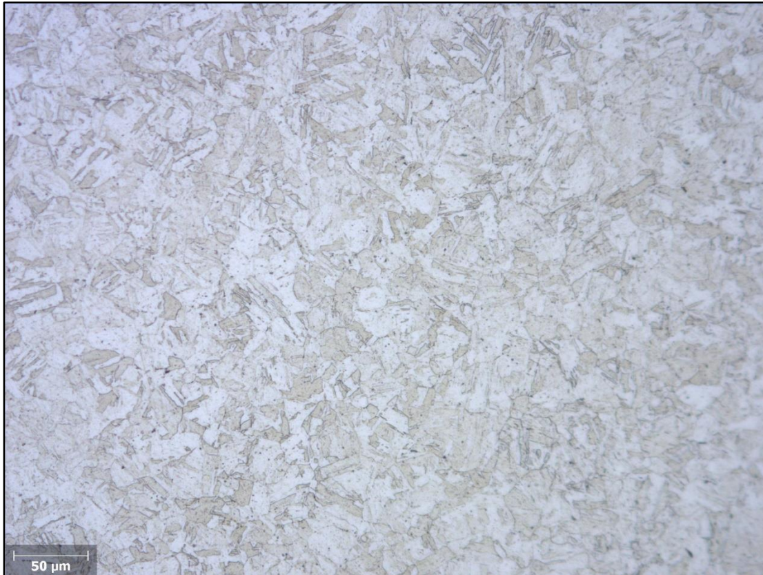
Figure 14: The microstructure after etching with Adler for 3 seconds at core region – 200 x. Box B.
