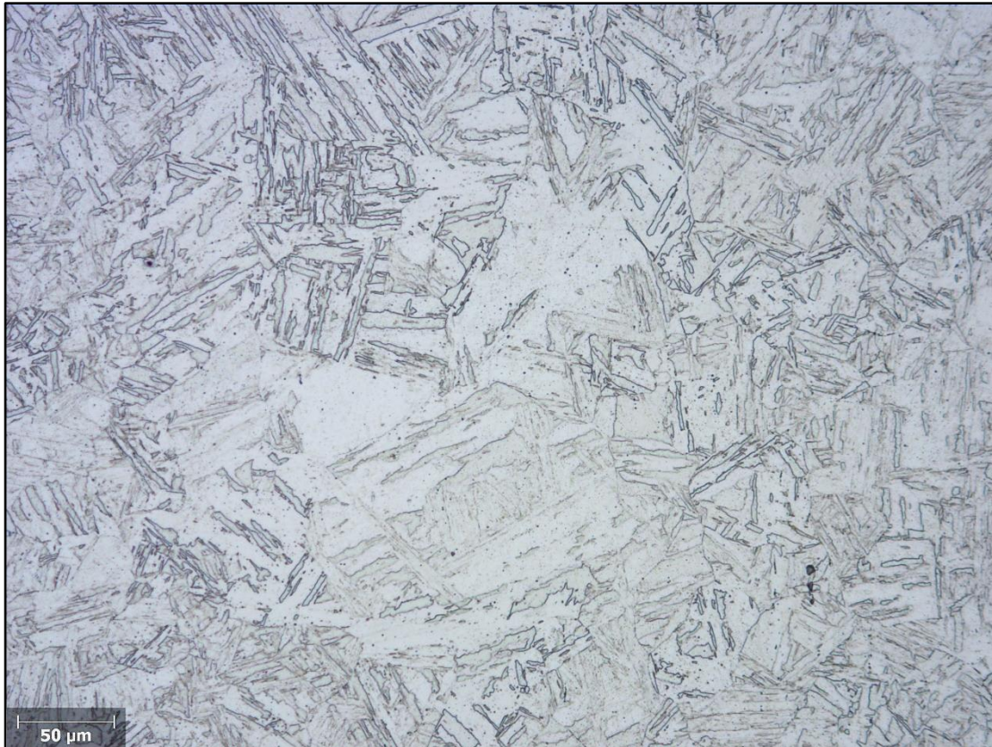
Figure 24: The microstructure at the core region after etching – 200 x. Box B.
