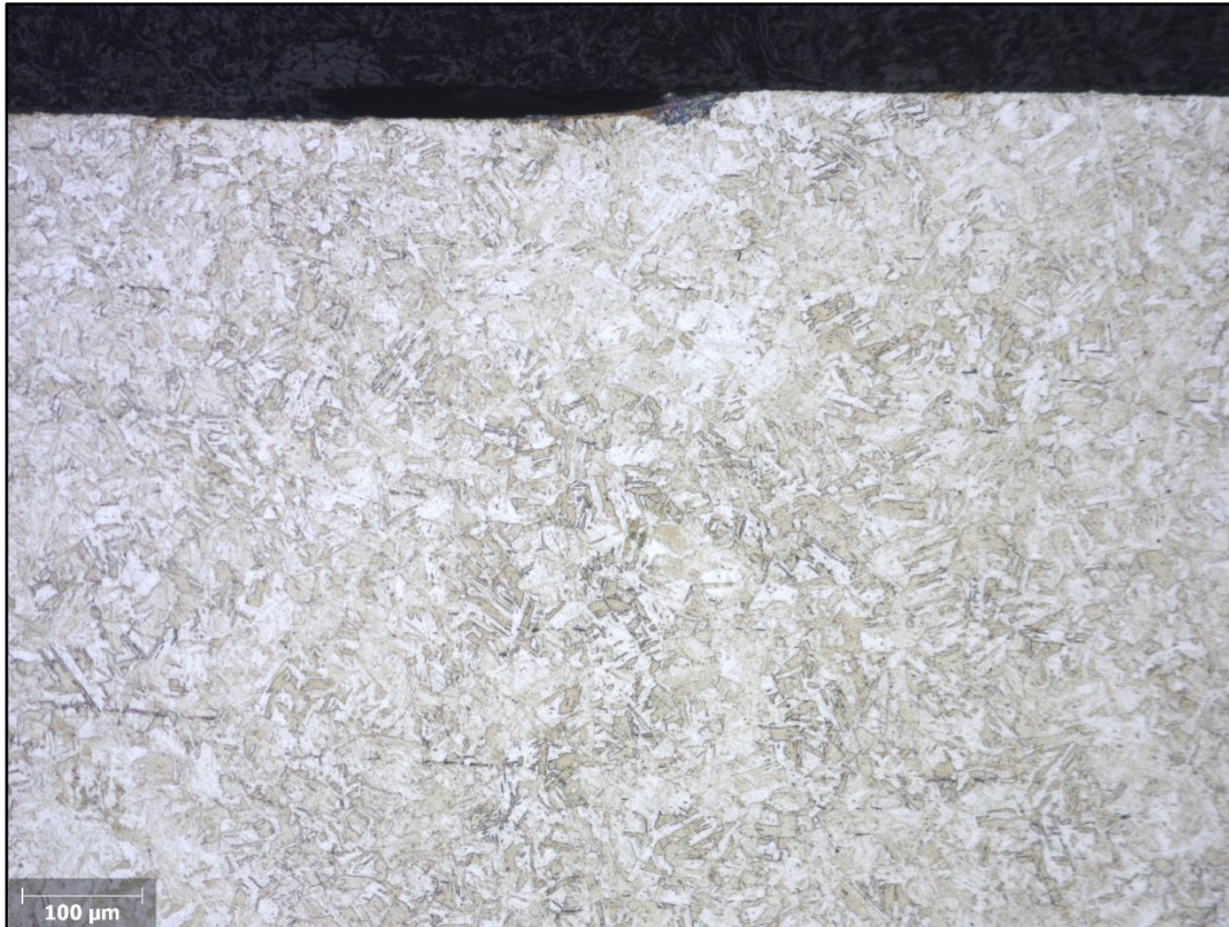
Figure 12: The microstructure after etching with Adler for 3 seconds – 100 x. Box B.
