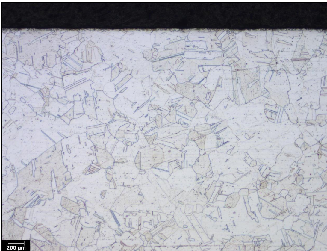
Figure 17: Microstructure after etching for 150 s with V2A at 50 °C - 25 x. Box A.
