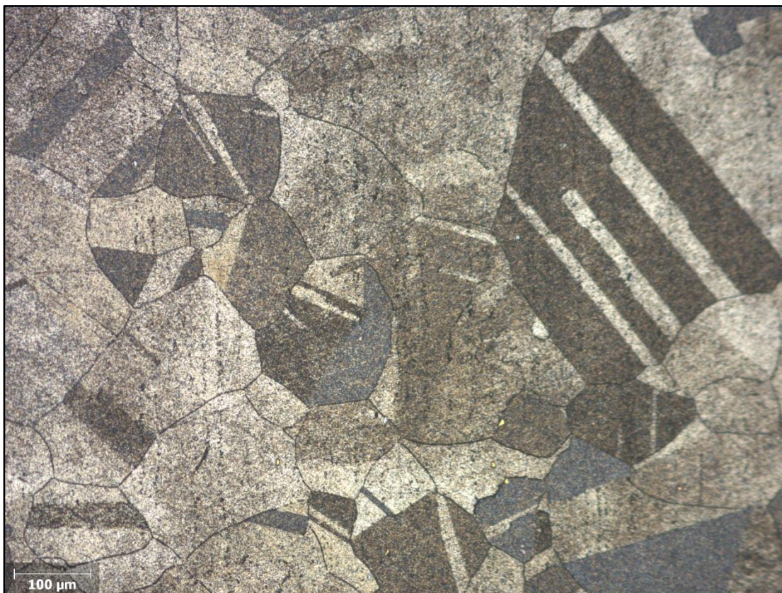
Figure 6: The microstructure after etching with Adler for 10 seconds – 100 x. Box A.
