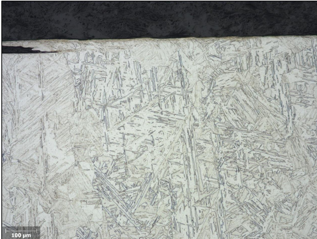
Figure 22: The microstructure of the sample after etching for 80 s with V2A at 50 °C – 100 x. Box B.
