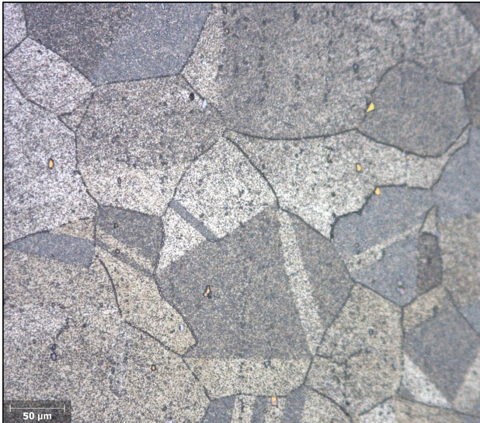
Figure 7: The microstructure after etching with Adler for 10 seconds – 200 x. Box A.
