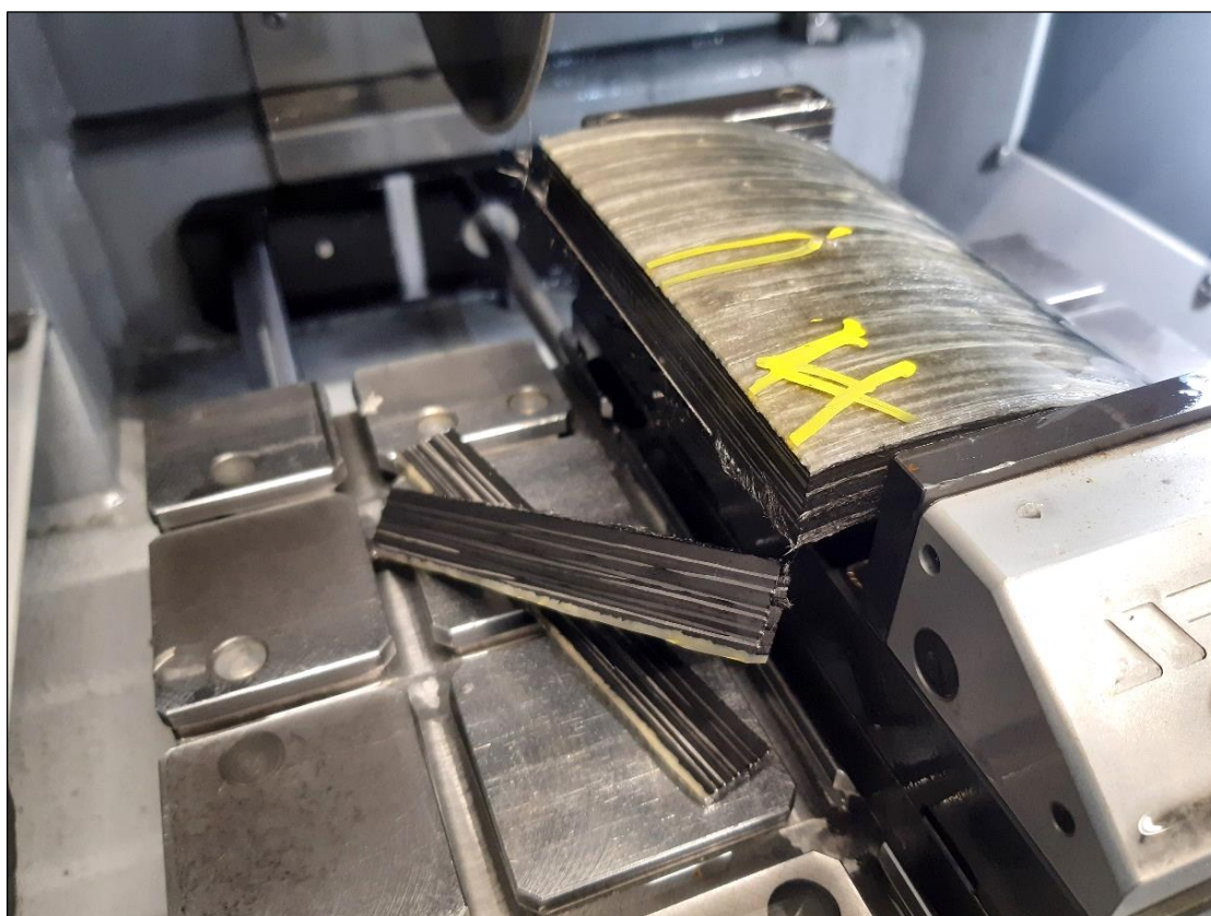
Figure 3: The sample after first two cuts X-Axis.
