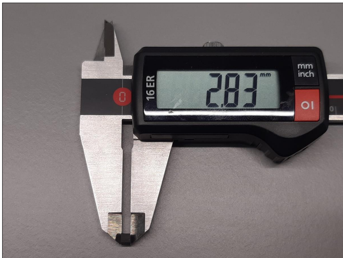
Figure 8: Cut sample measured with MarCal 16 ER caliper.
