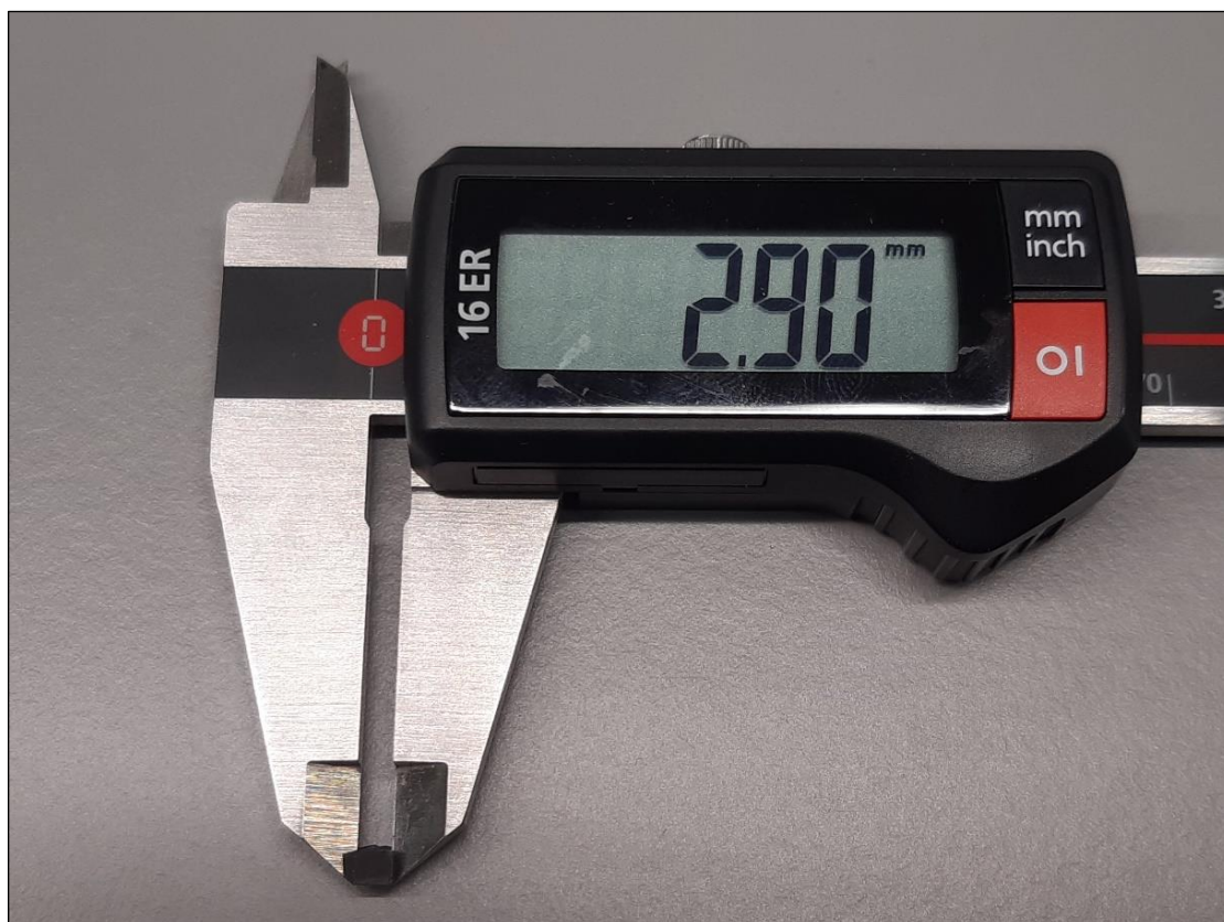
Figure 9: Cut sample measured with MarCal 16 ER caliper.
