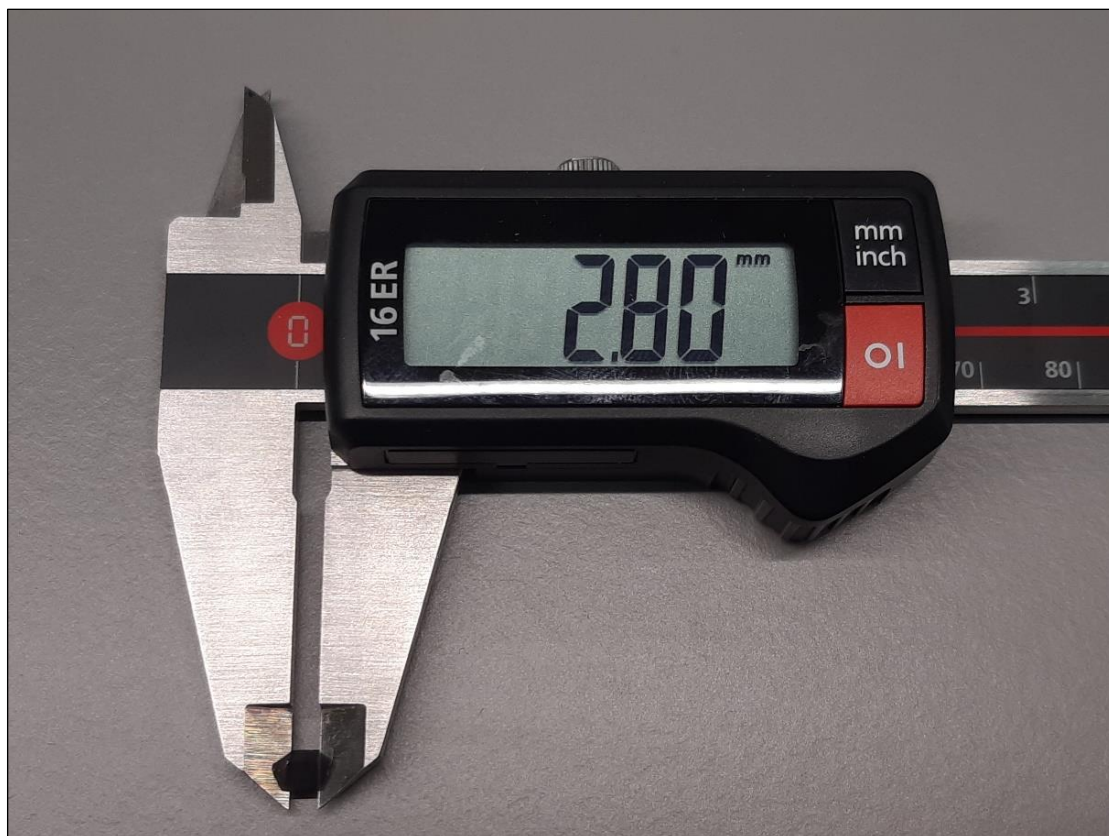
Figure 10: Cut sample measured with MarCal 16 ER caliper.
