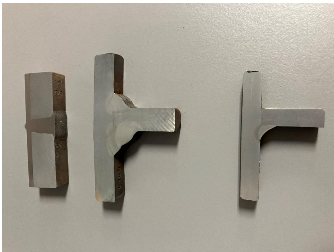
Figure 4: 3 small samples after etching with nitric acid 3%.
