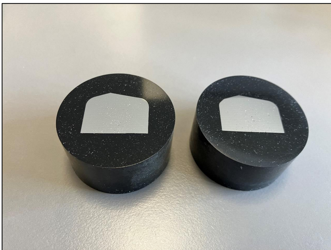
Figure 8: Parts 2 and 3 of sample A in figure 5 after mounting.
