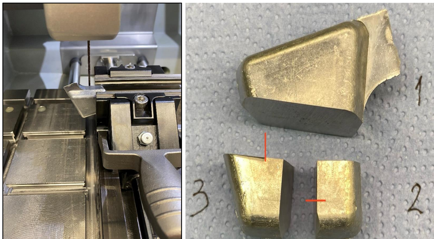
Figure 7: The cutting layout of sample A and different parts after cutting.
