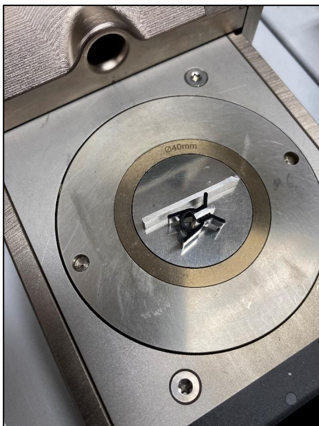
Figure 15: The cut samples were mounted in cross-section and lengthwise.
