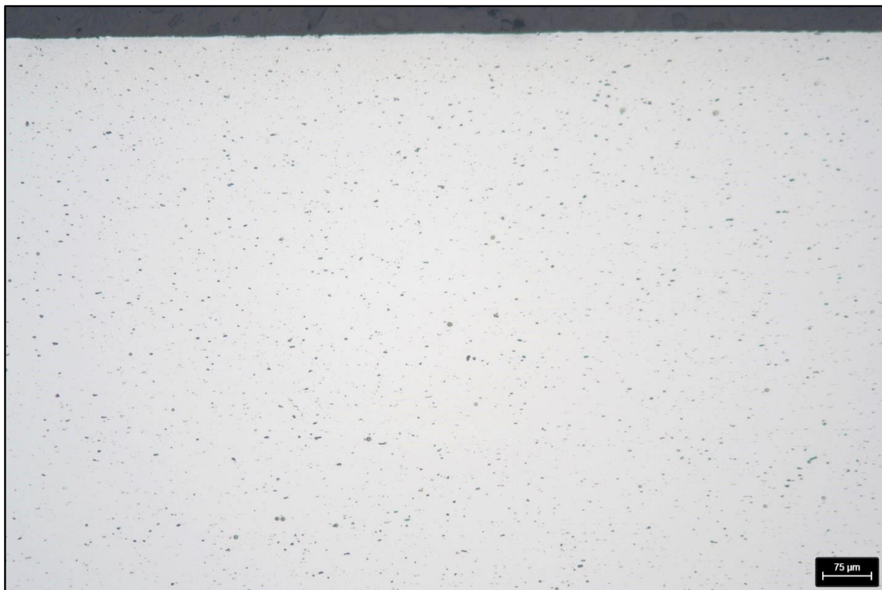
Figure 16: The Ext-Water sample after 1 µm polishing, not etched – 100 x
