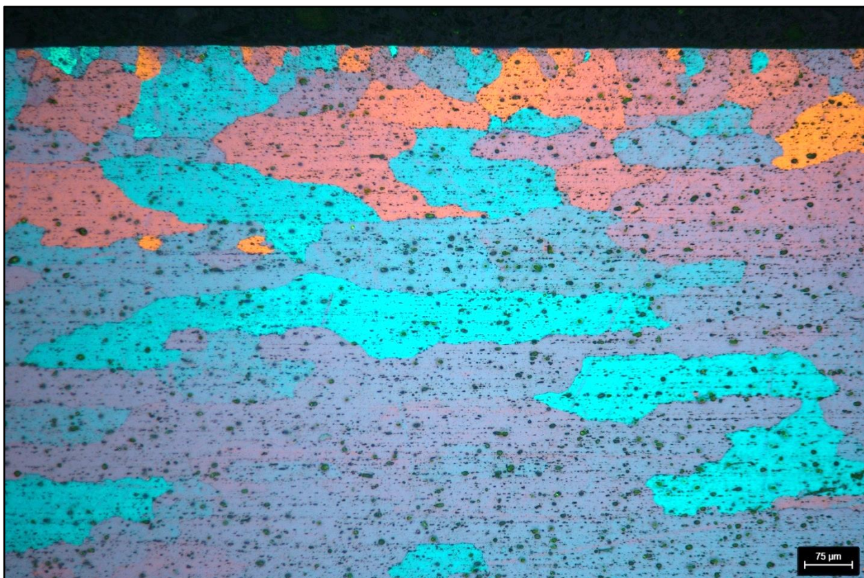
Figure 21: The Ext-Water sample after normal grinding/polishing and electrolytic etching – 100 x
