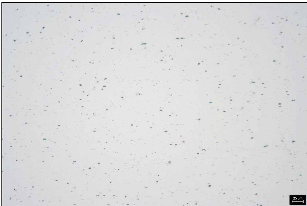
Figure 17: The Ext-Water sample after 1 µm polishing, not etched – 200 x
