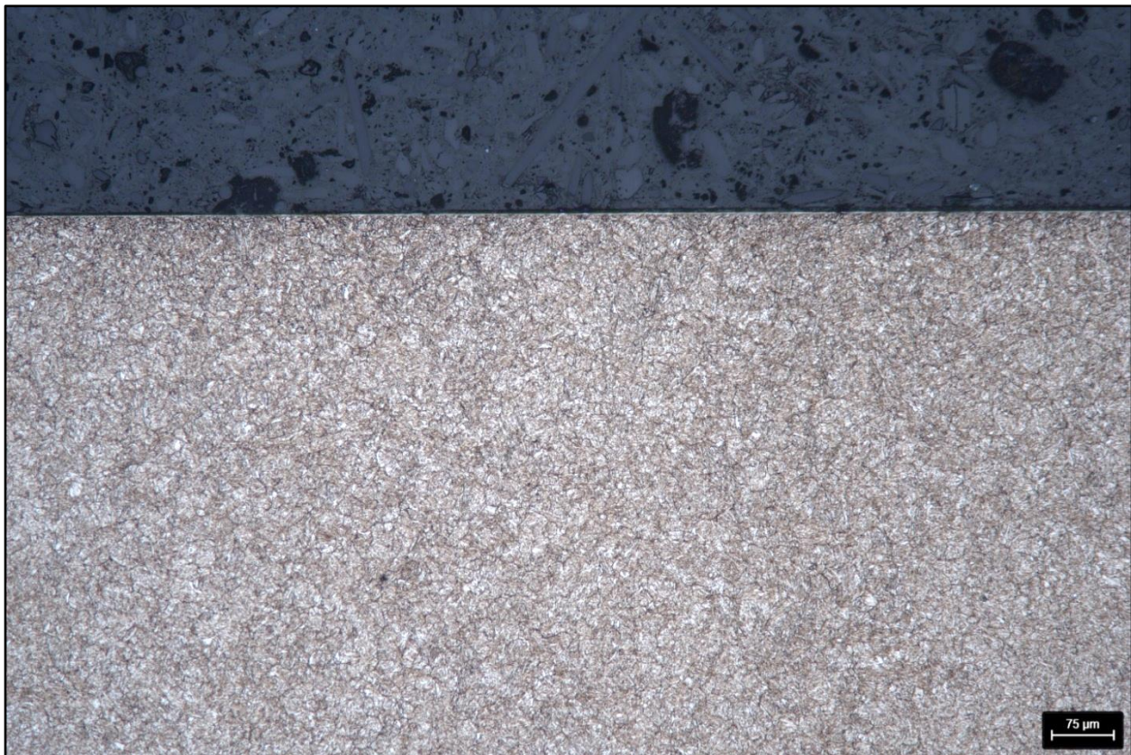
Figure 3: The nitride coating after etching under optical microscope – 100 x
