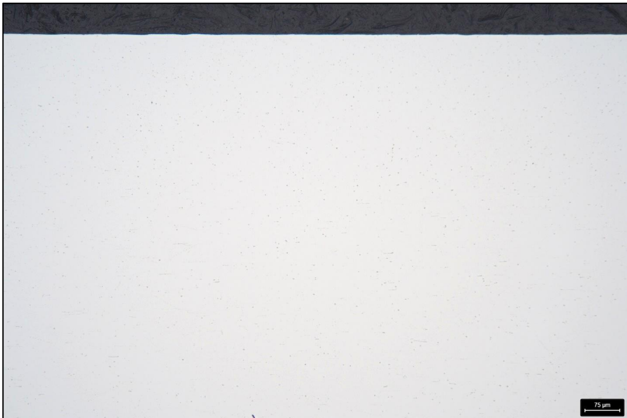
Figure 8. Sample 2 after fine polishing on the edge area – 100:1
