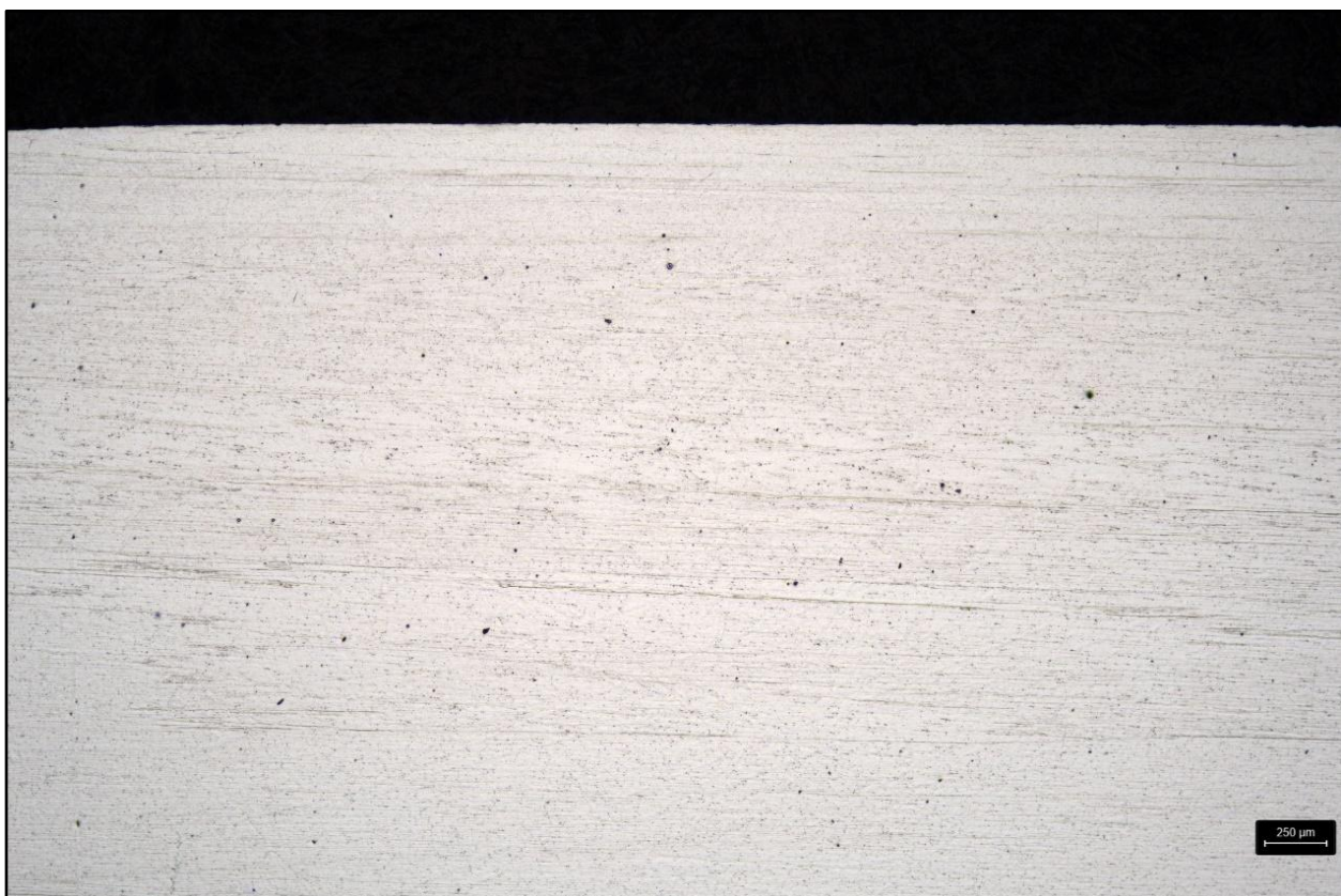
Figure 11. Sample 2 after etching for 4 minutes – longitudinal section - 25:1
