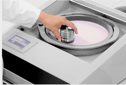
Inserting the mounted sample
