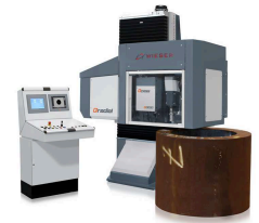
Milling and hardness testing position
