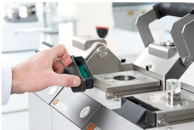
3. Clean dirt trap as excess mounting material is automatically pushed towards it
