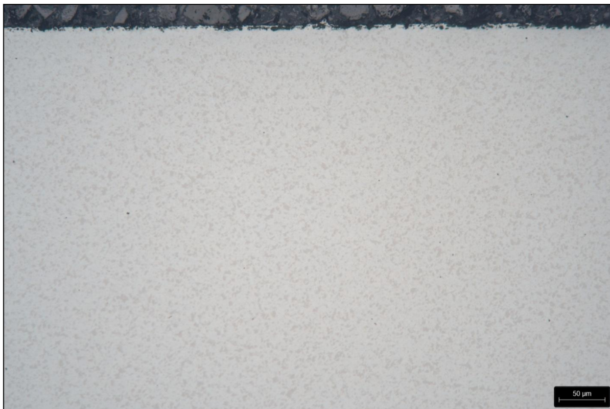
Figure 9. Sample A after fine-polishing with Eposil F without primary etching – 200 : 1
