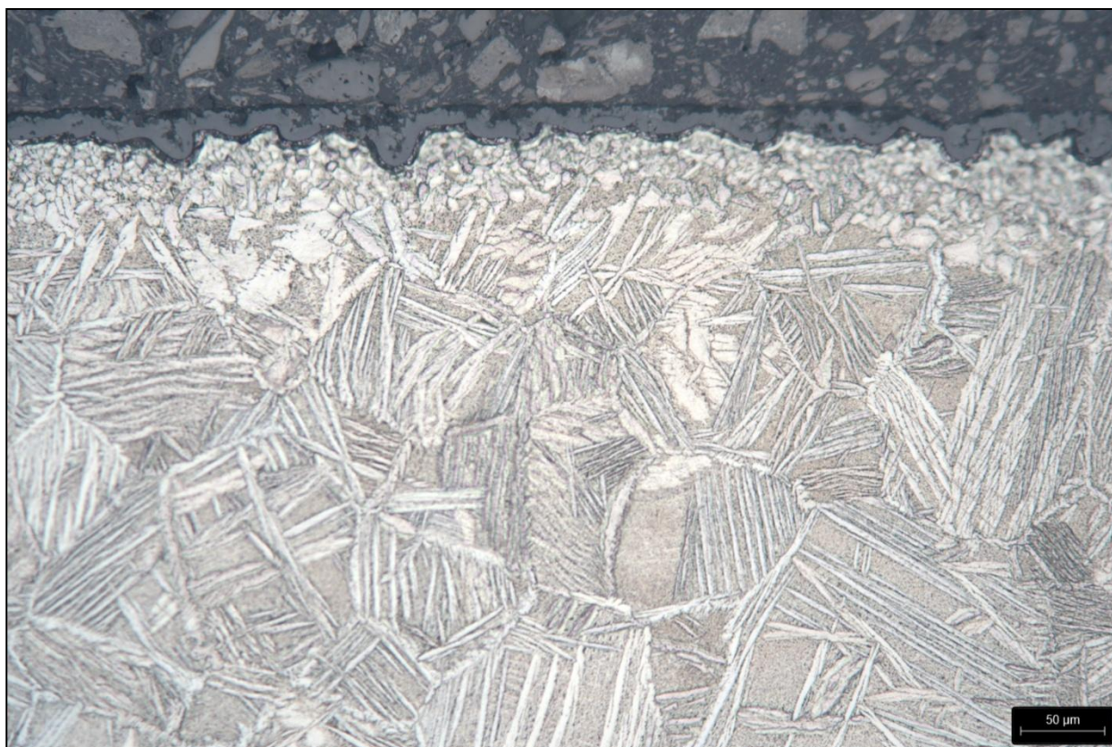
Figure 4. Sample 8F after fine-polishing with Eposil F and etched with Kroll – 200 : 1
