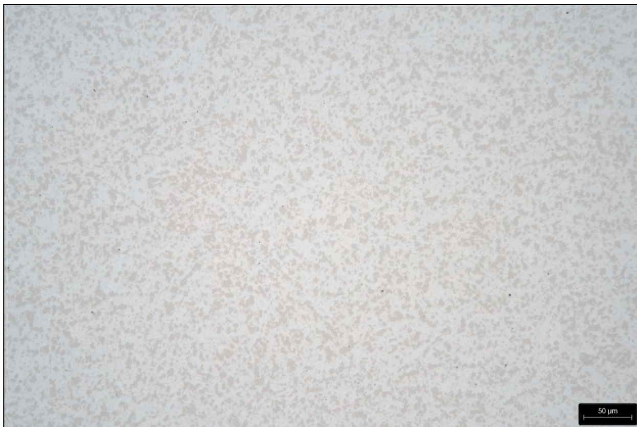
Figure 5. Sample 8F after fine-polishing with Eposil F and without primary etching – 200 : 1
