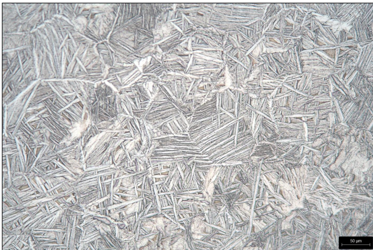
Figure 6. Sample 8F after fine-polishing with Eposil F and etched with Kroll – 200 : 1
