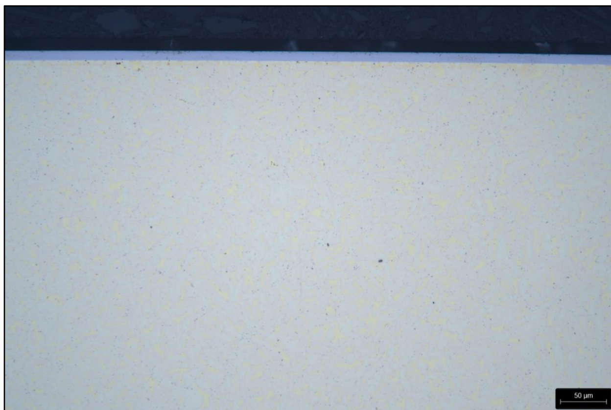
Figure 11. The coated samples after fine polishing – 200:1
