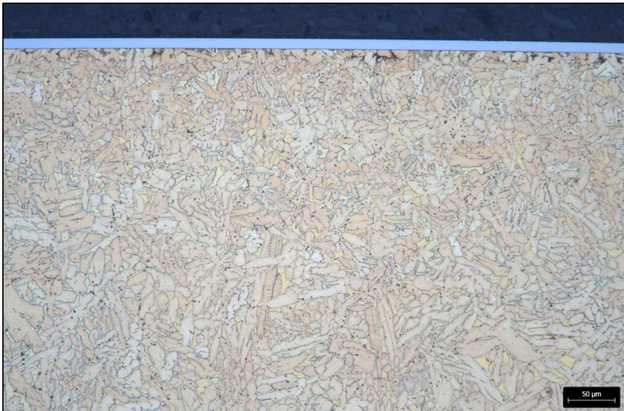
Figure 12. The coated sample microstructure after etching – 200:1
